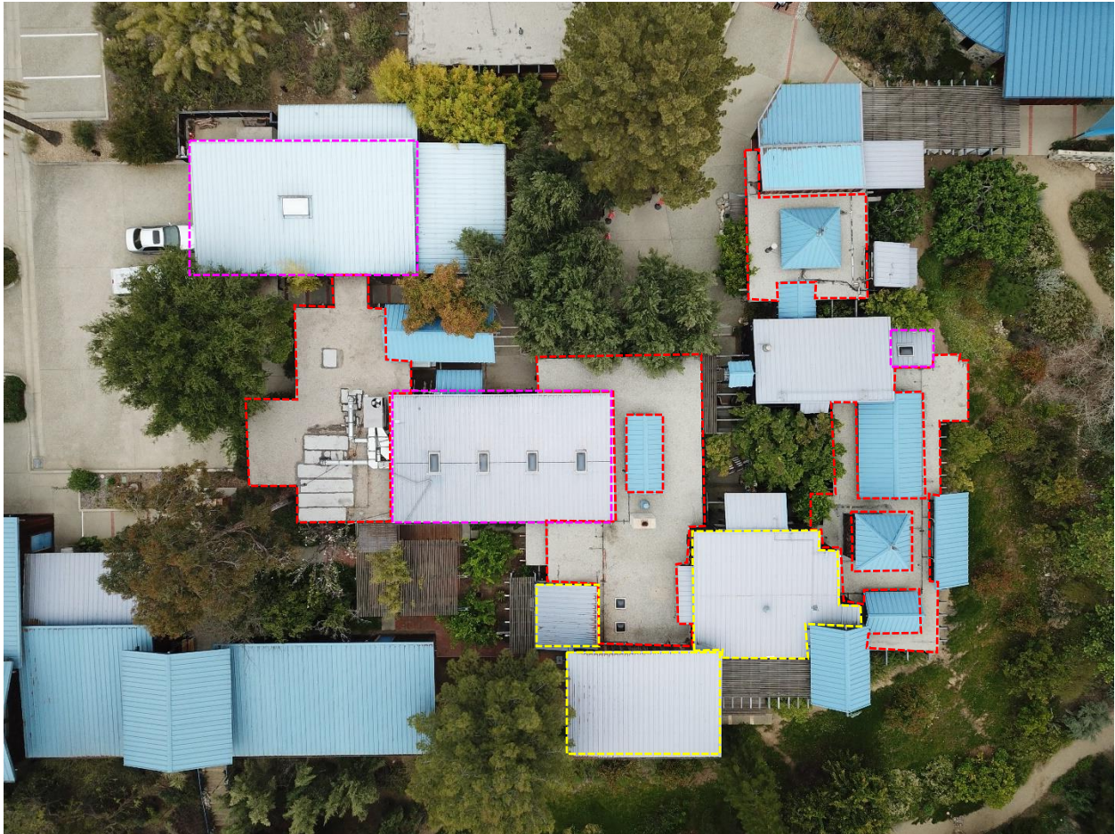
Figure 18. Aerial image of complex with flat roofs shown to be replaced with dashed red boundary lines and metal roofs to be replaced with magenta dashed boundary lines. Roofs with yellow dashed boundary lines are currently designated as alternate roofs for consideration of replacement based on poor insulative performance.
