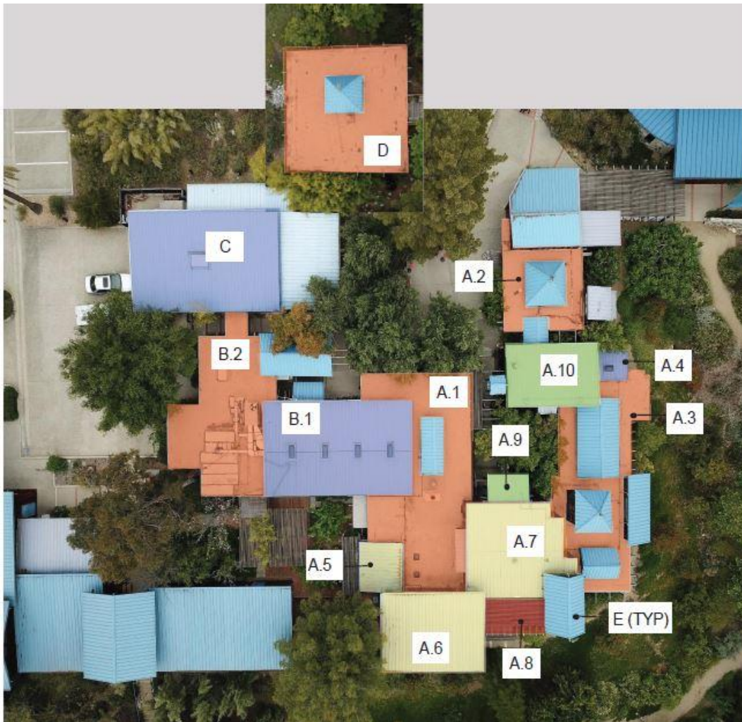
Image 1: Aerial image of Maloof Compound proposed repair and replacement of roofs. Refer to Attachment C Maloof Table for roof code, location, proposed roof types, recommendations, and comments. Orange indicates flat roofs to be replaced, purple indicates metal roofs to be replaced, red indicates south balcony to be replaced, yellow indicates metal roofs that are additive alternate (high priority), green indicates metal roofs that are additive
